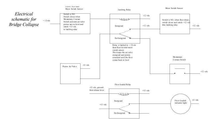
Depending on completed construction, the 'ground' for the Floor Load indicator lamp could come direct from the release lever making contact with the pivoting floor section. In order for this to work, all sections of the bridge must be isolated from electrical ground. The pivoting section is then grounded to a 12vdc power source and a wire is attached to the end of the release lever. When contact is made the light illuminates.
