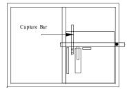
release lever is ½" thick steel 1 ½" wide approximately 28" long. The pivot bolt is plywood flooring is counter sunk for the Double nut the end of the bolt. The must move easily. A capture bar placed return spring and air piston will keep the from sagging and will hold it against the
